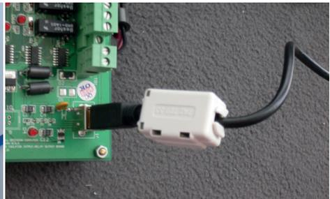
Folding core on the USB cable to the USB IO
