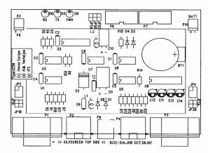
The xCON converter contains a few blocks of jumpers (switches) to configure the converter.
