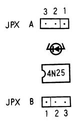
JPOB to JP7B are used to select isolated or non-isolated. When JPXB-1, JPXB-2 is sort, then the corresponds channel is in isolator mode. When JPXB-2, JPXB-3 is short, the IxL is short with system Gnd. So the external signal is in non-isolated mode. JPOA to JP7A are used to select power signal input or non-power signal input for the correspond channel. JPxA-1 and JPxA-2 short is power signal input mode. JPxA-2, JPxA-3 short is non-power input mode.
